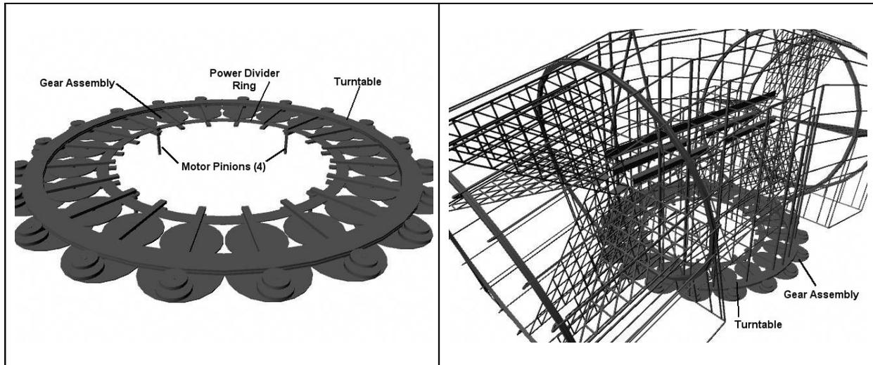
Figure 7. Turntable and Gear Assembly
