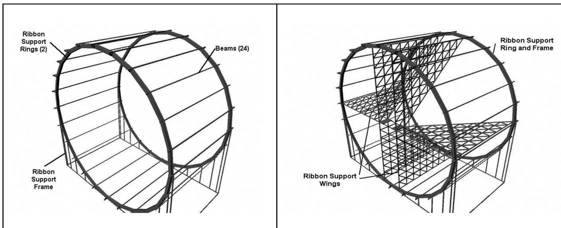
Figure 4. Ribbon Support Ring and Frame
